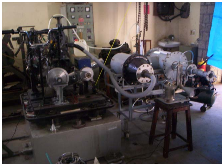
Figure 2. Picture of the experimental setup used in conducting the engine experiments with biogas. The airflow and fuel flow measurement rigs are also shown.
